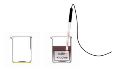
6. Pour the diluted iodine solution into the beaker containing the vitamin solution and observe the color change.
